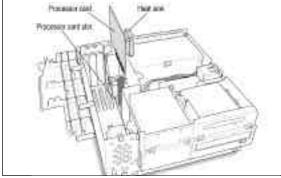
Removing the CPU card from a PowerMacintosh 7300
